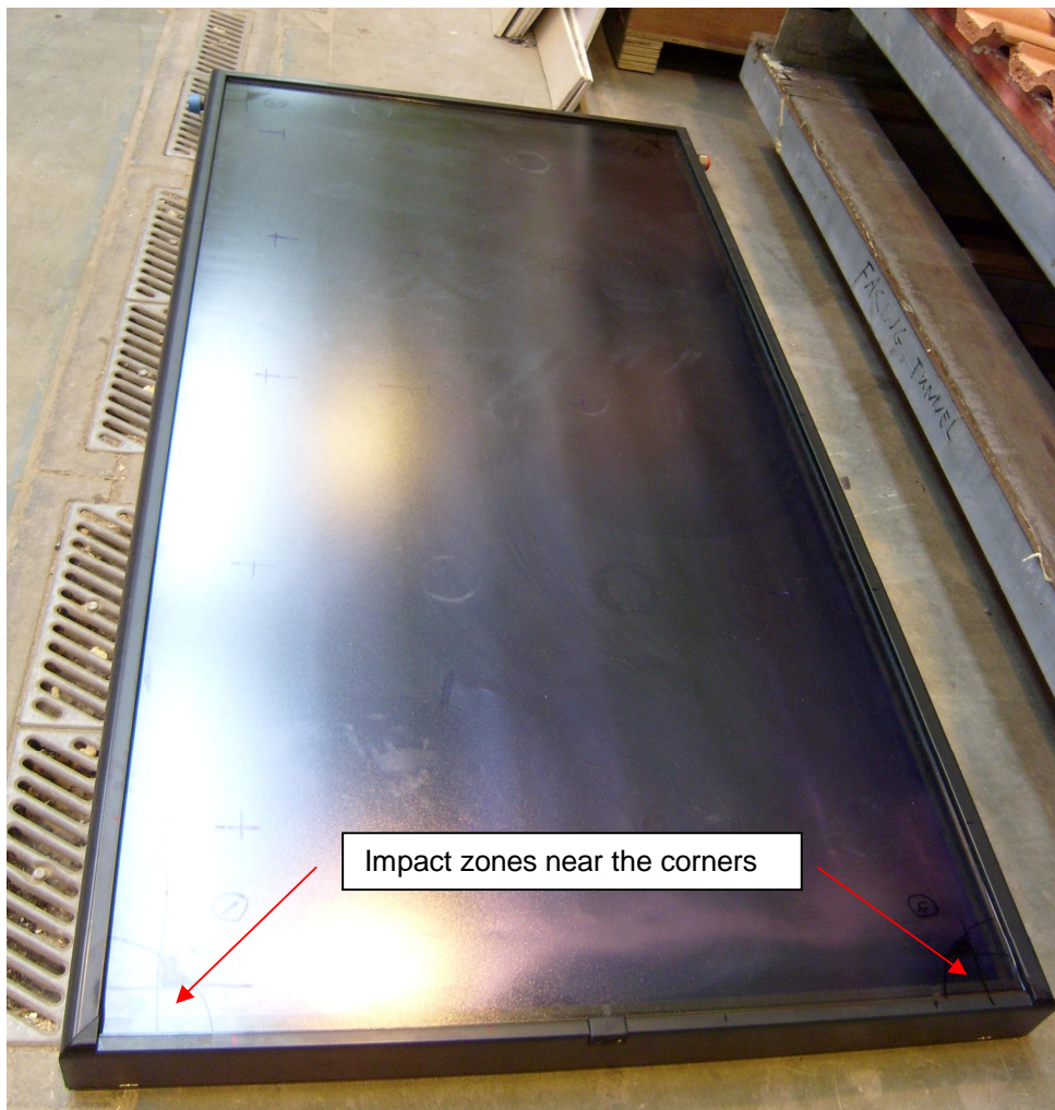
Figure 8 View of the collector after all impact testing has been completed
